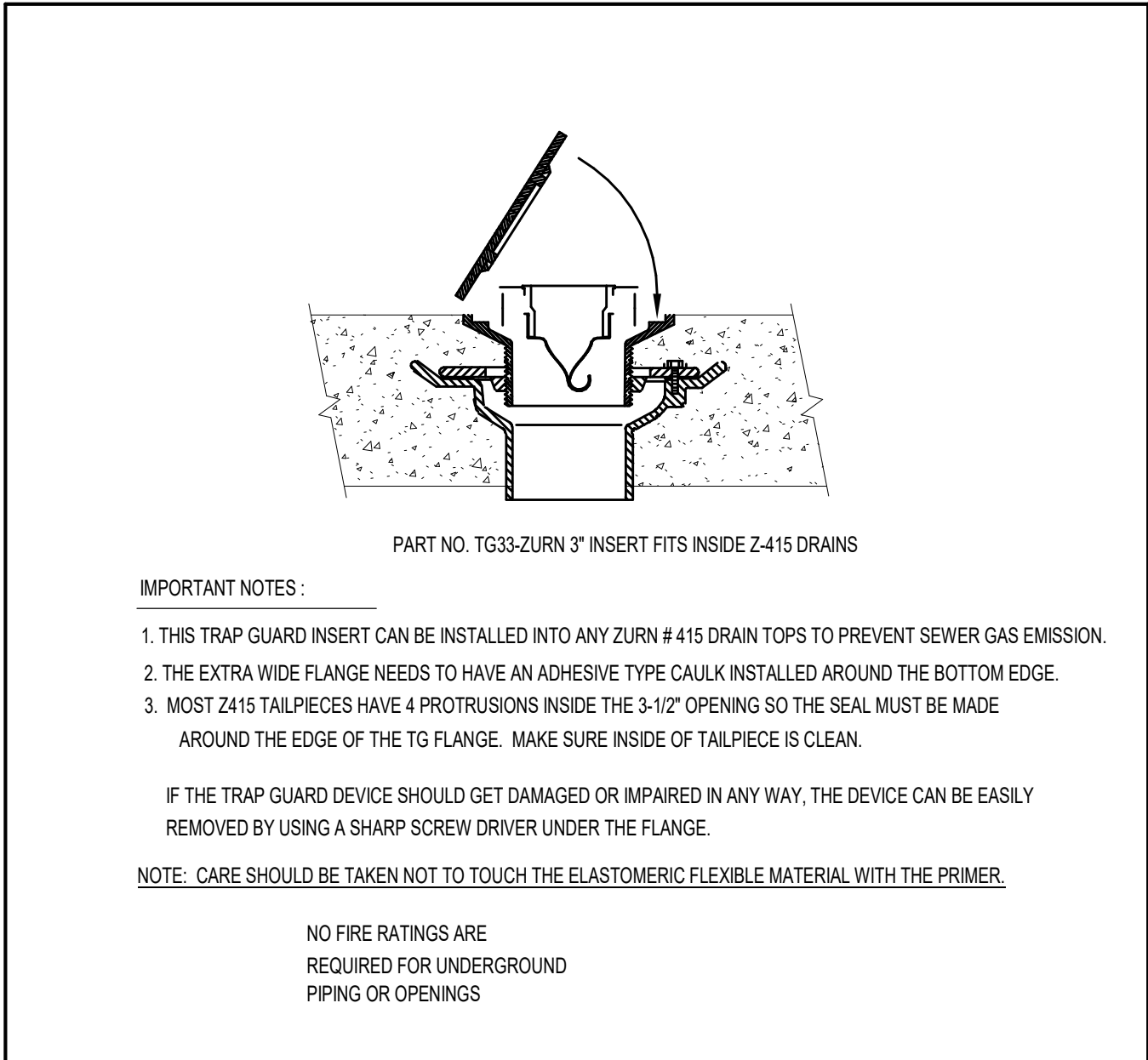
6 TRAP GUARD INSERT DETAIL NOT TO SCALE
